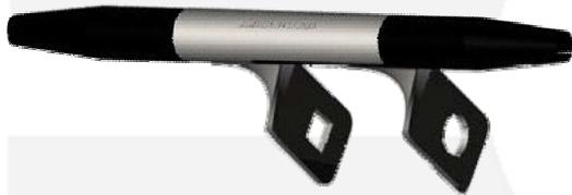
The cable support now features a round hole on one side and a square hole on the other. The assembly of the intermediate passing point shaft in one hole or the other governs how it is used (fixed or mobile passing point).
