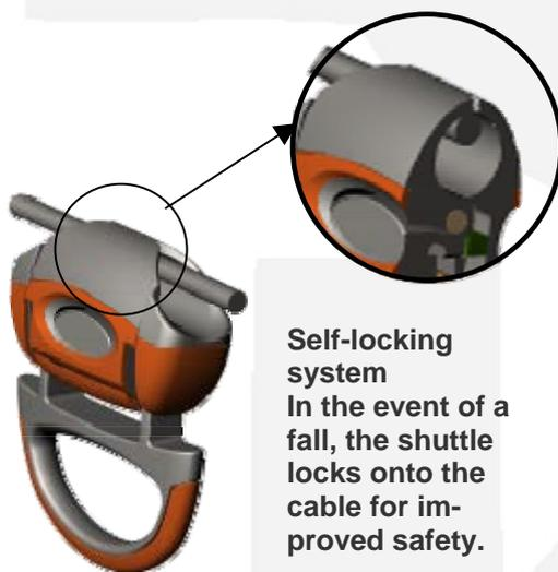
The free patented connection ring allows the user to work on both sides of the lifeline without having to unfasten or turn the shuttle. This is very useful for lifelines which are installed on roofs, ridgelines, or under the ceiling.
