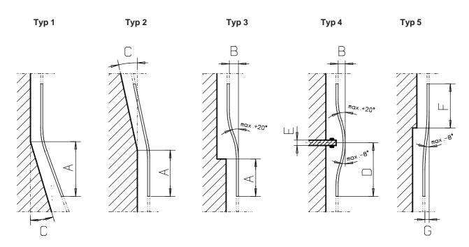
A = Bottom edge of ladder to salient point of structure
